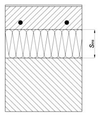
Fig. 4.7. Cross-section through a traditional floor heater with non-profiled thermal insulation [17]
