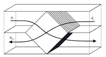
Fig. 2.9. Heat recovery by a plate heat exchanger [3]
