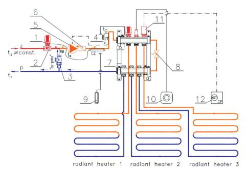
Fig. 4.23. Temperature control system of radiant heating with multiple heating circuits [30]:
