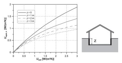
Fig. 2.7. Equivalent heat transfer coefficient of a heated basement wall — based on [1]
