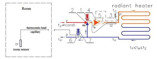
Fig. 4.15. Room air temperature control system with thermostatic head and capillary [26]: 1 – thermostatic head with contact sensor, 2 – three-way mixing valve, 3 – safety switch, 4 – circulation pump, 5 – check valve, 6 – straight-way thermostatic valve, 7 – thermostatic head with room sensor
