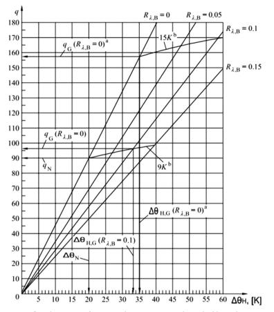
Fig. 4.6. In-floor heating performance characteristics, with marked boundary curves [16]; superscripts a and b indicate the edge zone and the boundary curve, respectively
