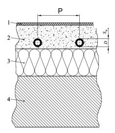
**Fig. 4.4.** System with under-screed ducting (type B) [16]; 1 – floor covering  $(R_{\lambda,B})$ , 2 – screed  $(\lambda_E)$ , 3 – heat conducting element, e.g. steel sheet, 4 – insulation layer, 5 – structural base
