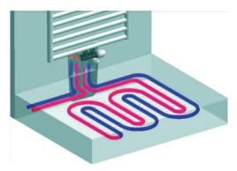
Fig. 4.44. Connection unit with floor heater [29]
