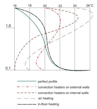
Fig. 4.1. Temperature profile for various heating types [12]
