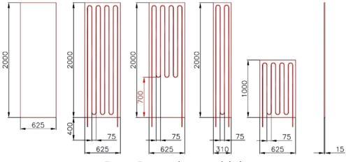
Fig. 4.29. Dry system heating panels [29]
