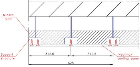
Fig. 4.33. Dry system ceiling heating [29]
