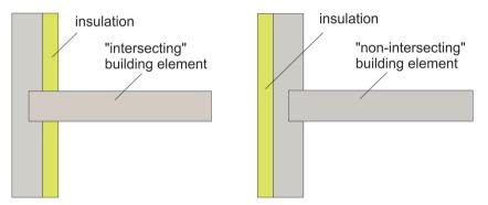
Fig. 2.3. Insulation "intersecting" and "non-intersecting" building elements [1]
