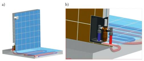
Fig. 4.40. In-floor heating control system with double temperature adjustment [29]; a) control system components, b) Floor Fix unit connection detail
