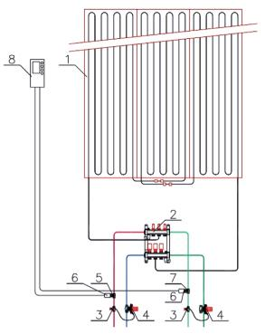
Fig. 4.34. Example of heating and cooling combined into one system [29]; 1 – wall panel, 2 – manifold, 3 – balancing valve, 4 – differential pressure regulator, 5 and 7 – thermostatic valves, 6 – thermal actuator, 8 – controller
