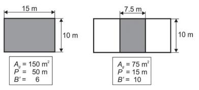
Fig. 2.8. Determination of characteristic dimension B' [1]
