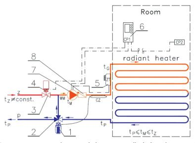
Fig. 4.21. Room temperature control system with electronic controller [28]: 1 – thermostatic head with contact sensor, 2 – three-way isolation valve with minimal bypass, 3 – straight-way thermostatic valve, 4 – thermal actuator, 5 – safety switch, 6 – room controller, 7 – circulation pump, 8 – check valve
