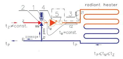
Fig. 4.13. Thermostatic temperature control system with a three-way valve at feed [24]: 1 – thermostatic head with contact sensor, 2 – three-way mixing valve, 3 – safety switch, 4 – circulation pump, 5 – check valve
