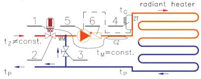
Fig. 4.9. Thermostatic temperature control system with a straight-way valve [20]:
