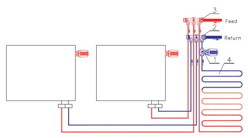
Fig. 4.38. Floor comfort system with panel radiators with incorrect RTL connection [34];
