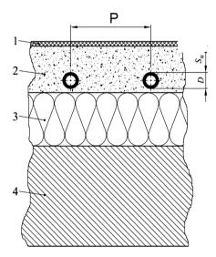
**Fig. 4.3.** System with in-screed ducting (types A and C) [16]; 1 – floor covering  $(R_{\lambda,B})$ , 2 – screed  $(\lambda_{E})$ , 3 – insulation layer, 4 – structural base
