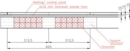
Fig. 4.32. Dry system in-floor heating [29]
