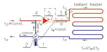
Fig. 4.11. Thermostatic temperature control system with a three-way valve at return [23]:
