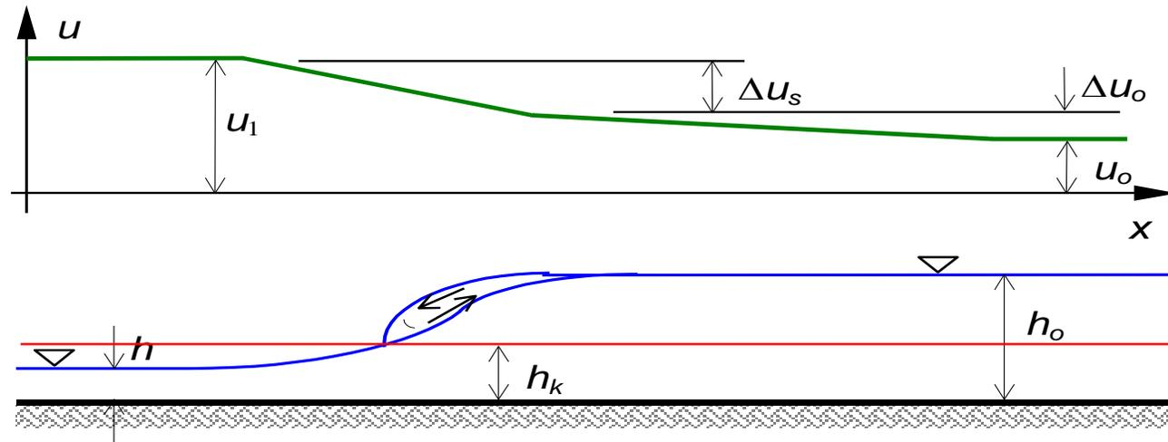
The form and characteristics of the hydraulic jump depend upon both depths  $h$  and  $h_o$  – which are known,
