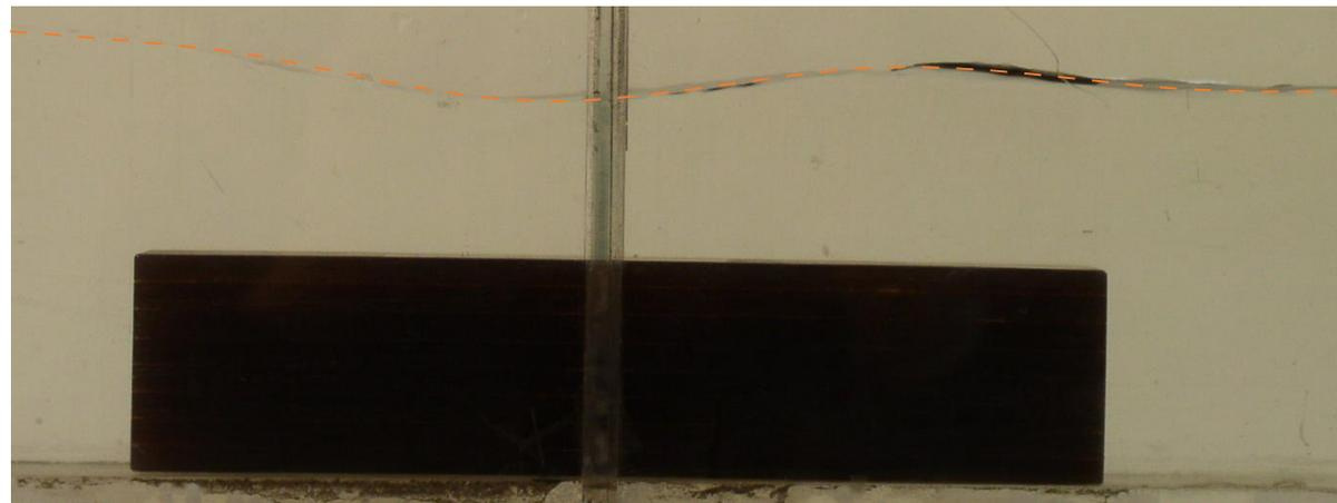
Shape of water profile in the case of submerged weir
