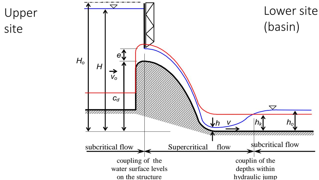
When water flows through the damming construction, depth changes occur:
