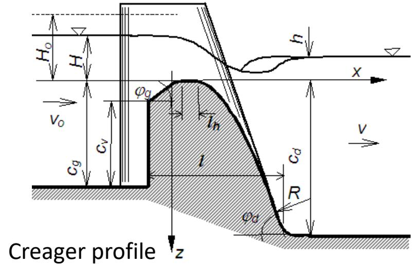
The required degree of submergence to reduce discharge of weir by tailwater  $\left( \frac{H - h}{C_d} \right)_k$
