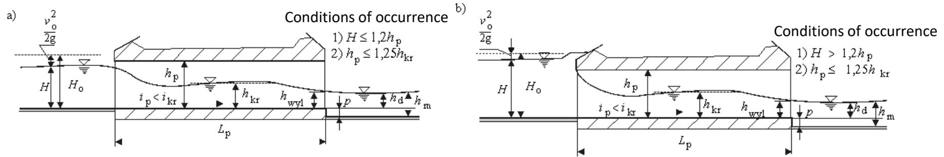
Free flow with unsubmerged entrance free flow with submerged entrance
