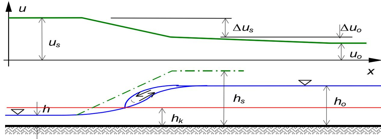
To assess whether the hydraulic jump is submerged, the submergence criterion is required:
