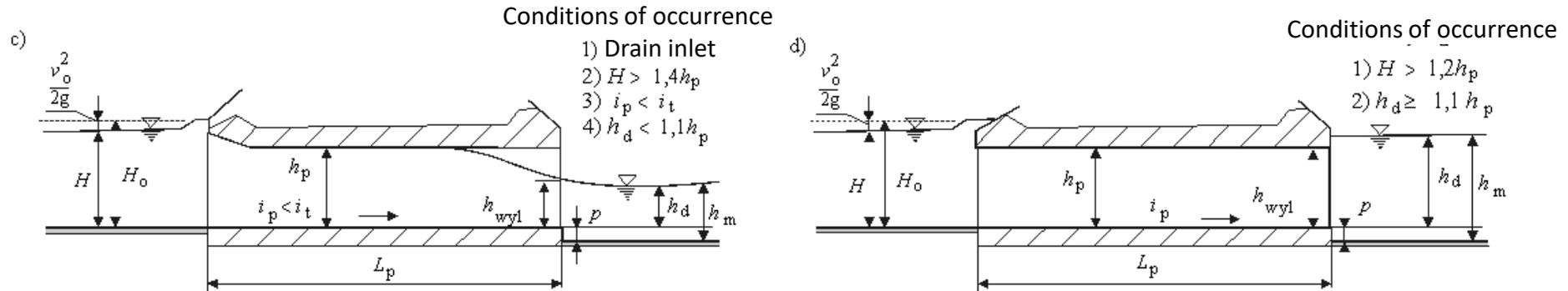
Pressurized flow with unsubmerged outlet pressurized flow with submerged outlet
