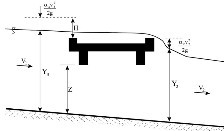
Overflow of bridge and pressure flow below the bridge
