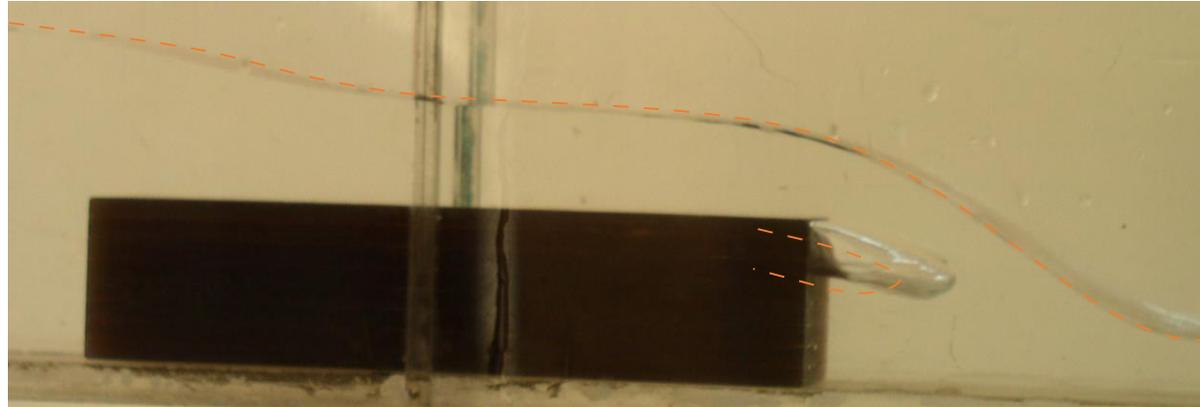
Shape of water profile in the case of unsubmerged weir
