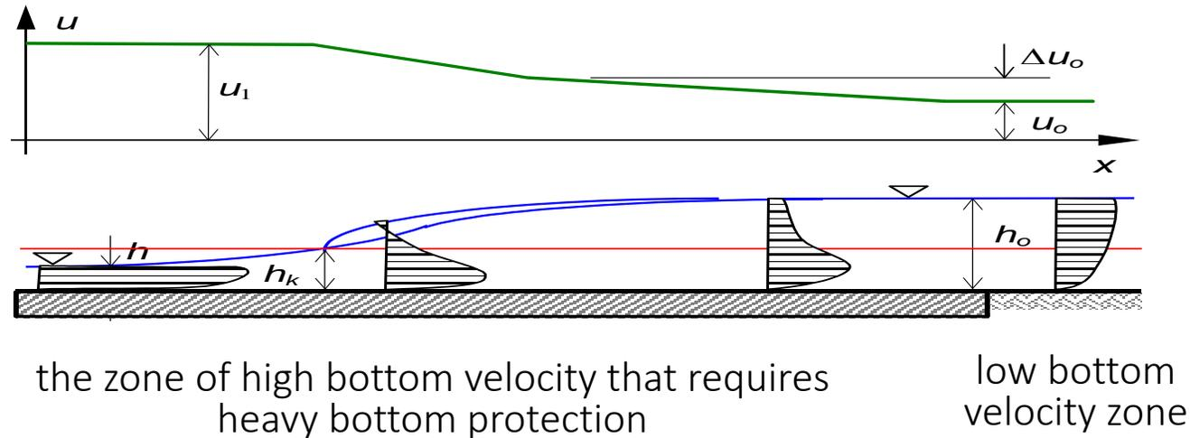
Unsubmerged hydraulic jump should be avoided downstream of the hydraulic structure because:
