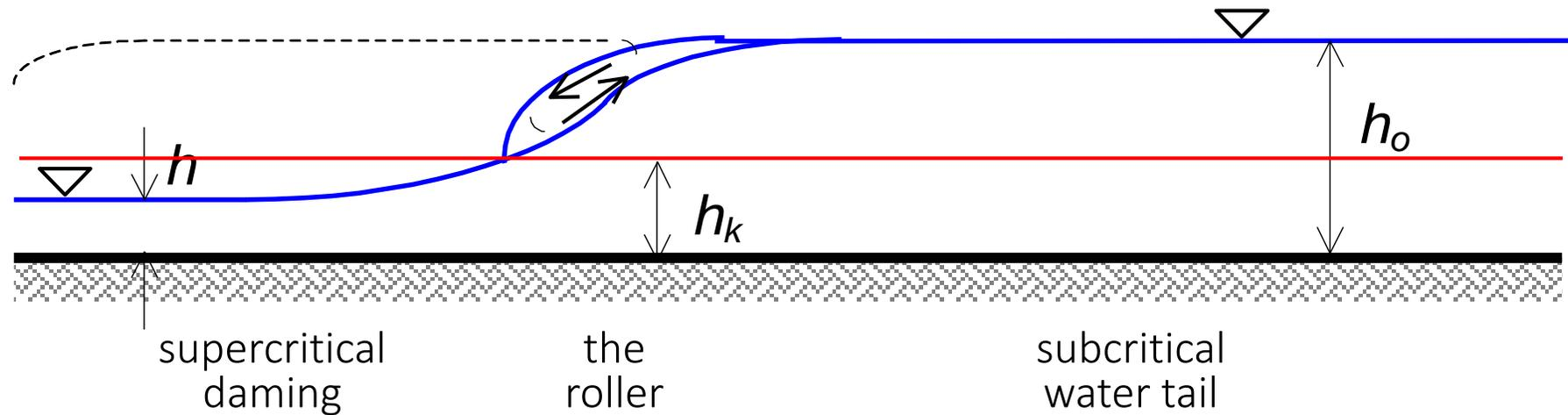
In the lower station, there is a transition from the subcritical depth  $h$  to the normal depth  $h_o$  in the outflow channel:
