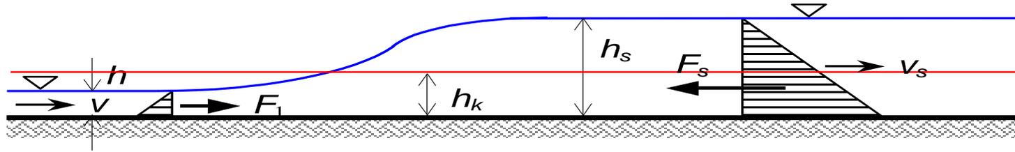
The force impulse is caused by the difference of hydrostatic force  $F_s - F_1$ :
